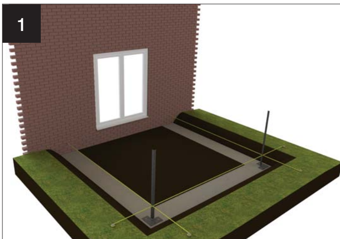
Using strings and timber pegs, set out for the masonry external leaf. Always check diagonal dimensions to ensure everything is square. Line up the outside edge of the set out post against the string lines – temporarily fix. Remove string lines, slide the set out post outwards by 3mm and then fix to concrete strip footing with the two anchor bolts provided.
