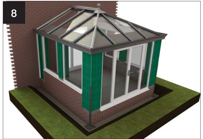
Install the Classic roof and Cornice in the usual way.
