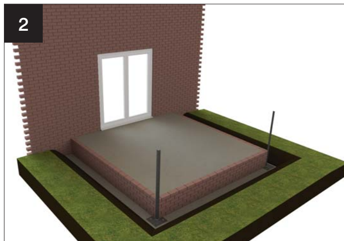
Build the masonry up to DPC level and concrete the slab in the usual way.
